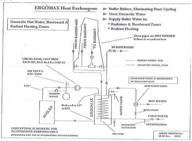
The dip tube is built into all models.
